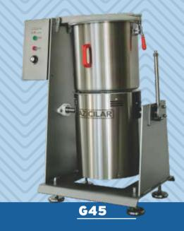
G20 is a vertical, standing, high capacity grinder with a 20 bowl and a straight blade knife G45 is a vertical, standing, high capacity grinder with a 45 bowl and a straight blade knife
